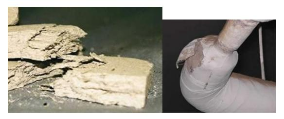
If any worker suspects that a material he is working on or is about to work on may contain asbestos, then they <u>MUST</u> stop work immediately and inform their supervisor so that further investigations may be carried out.
